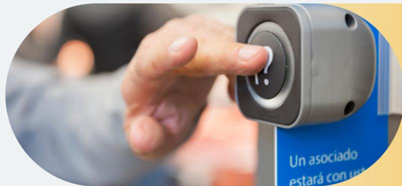
**Assistance button:** a wireless device connected to associates' portable radios that emits a predefined signal to request assistance in specific areas for people with disabilities.
